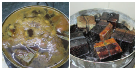
pieces were kept in Spent Wash Liquid at 100°C (hot Plate)
